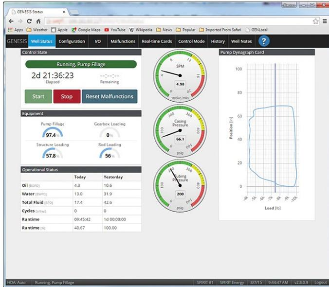
The Real-Time Card dashboard provides a wealth of operational analysis in graphical form, including real-time surface and pump dynagraphs that track the load on the rod and pump, and stroke statistics including the average strokes per minute and the volume of pump fillage as a function of its total capacity.
